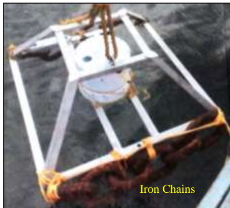
Fig. 3: Heavy iron chains tied below the base of the frame
