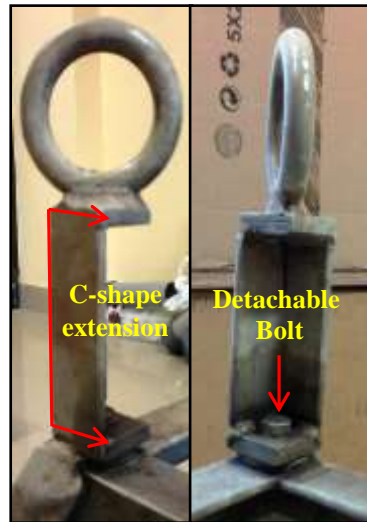
Fig.12a: Detachable Hook-loop assembly
