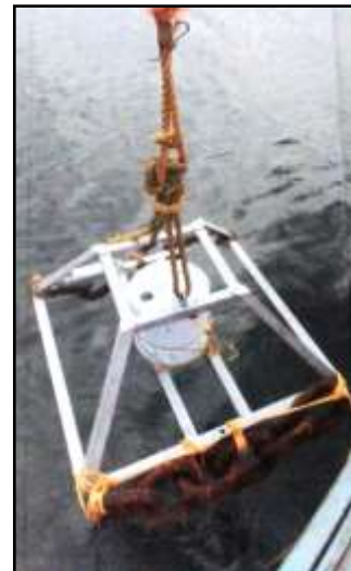
Fig. 5b: Deploying of Tide gauge with metal frame.
