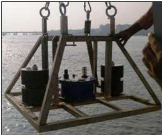
Fig. 15a: Tide Gauge & Counter weights mounted on the mooring frame
