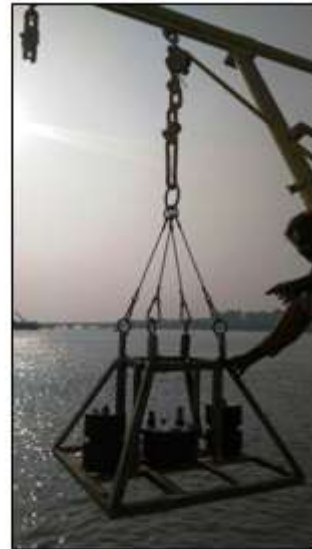
Fig. 15b: Tide gauge-in-Mooring frame deployment using SS wire ropes
