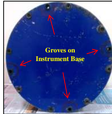
Fig. 11a: Drilled holes on frame & groves on tide gauge base
